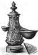
No. 215-A—Drinking Fountain. 5 ft. 4 in. high. Base 22 in. in diameter. For Man, Horse and Dog. Very heavy. Nae Basin supplied with Sanitary Bubbling Cup. Horse Basin supplied with ball cock regulating the flow of water.
