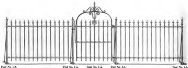
No. 41-A— \frac{3}{4} inch Round Pickets, spaced 4 inches on centers. 1\frac{1}{2} \times \frac{3}{4} inch Stewart Patent 3-Rib Channel Rail. Height from ground, when set, 37, 42 and 48 inches.
