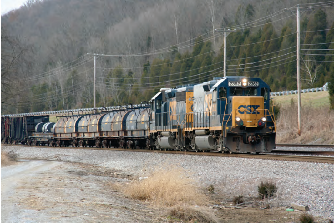
CSXT 2362, a Road Slug, and CSXT 6980, a GP40-2, leads a train of steel coil cars and empty metal waste gondolas from Gallatin Steel into McCormick Yard
